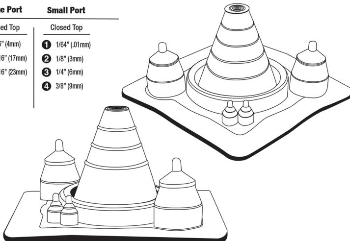
\* Find pipe size in table and trim Solar Multi-Port MR Master Flash® as shown on outline. \* Cut the flashing at least 20% less than the pipe Outer Diameter
